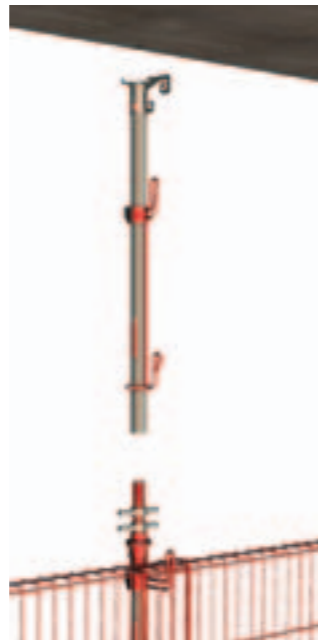
Step 4 Insert the extension post, placing the Soffit Grip on the top and fix onto the Compression Thread.
